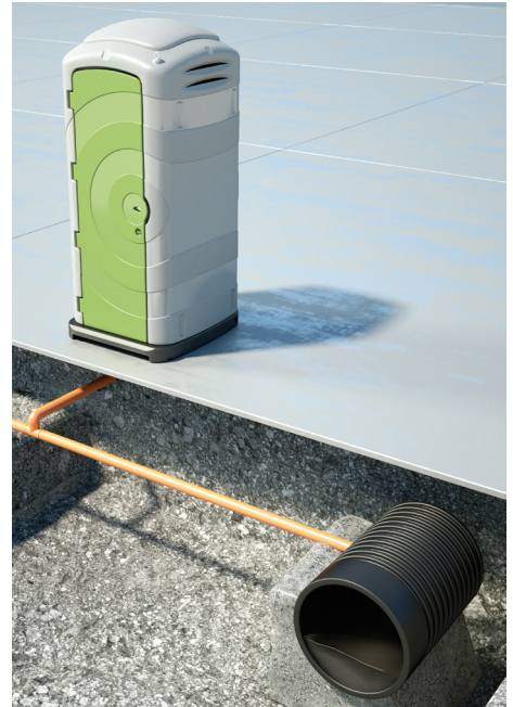
DISCHARGE TO PUBLIC SEWER
